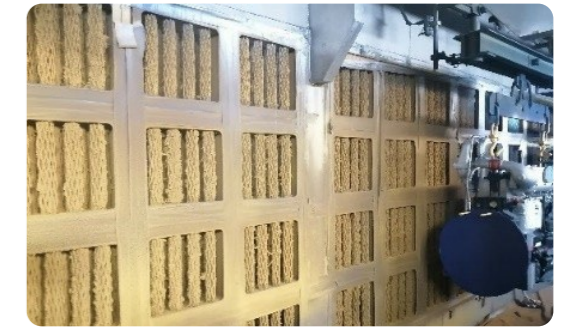
Renovating the dry spray booth to improve the adsorption and removal efficiency of spraying exhaust gas, reducing the concentration of emitted exhaust gases
