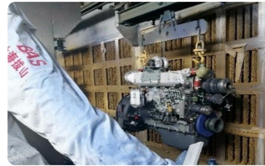
Renovating the dry spray booth to improve the adsorption and removal efficiency of spraying exhaust gas, reducing the concentration of emitted exhaust gases
